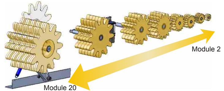
The gear lubricator segments are arranged onto a bushing. The bushing rotates around its mounting axle. The gear lubricator teeth meet precisely with the pinion drive teeth flank surfaces. A bore in the mounting axle supplies the lubricant to the gear lubricator outlets of the LUBCON LubeGearSystem.
