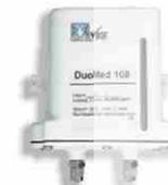
Double point lubrication unit for maintenance-free operation of e. g. electric motors up to a maximum of 3 years. It can also be used for fan shaft bearings and many others with a large variety of long life greases.
