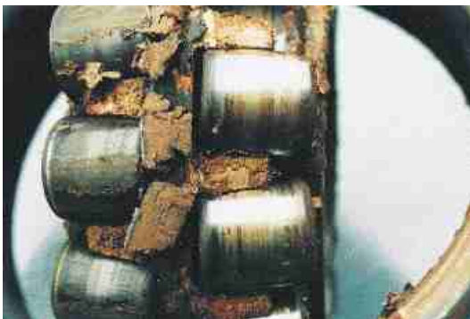
Fig. 3: Photos of roller tube surfaces as well as running tread of bearing inner ring - as tested see diagram 3, p. 6
